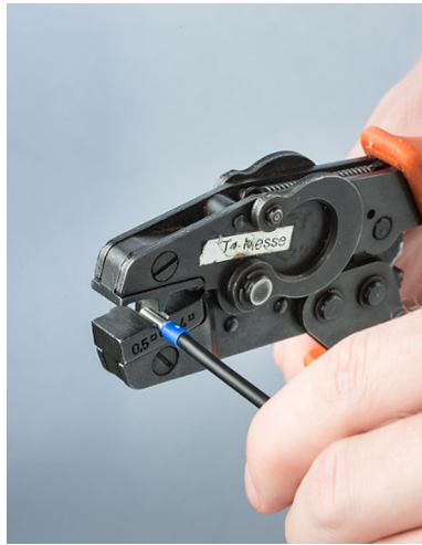
Figure 11-8 Manual crimping operation
