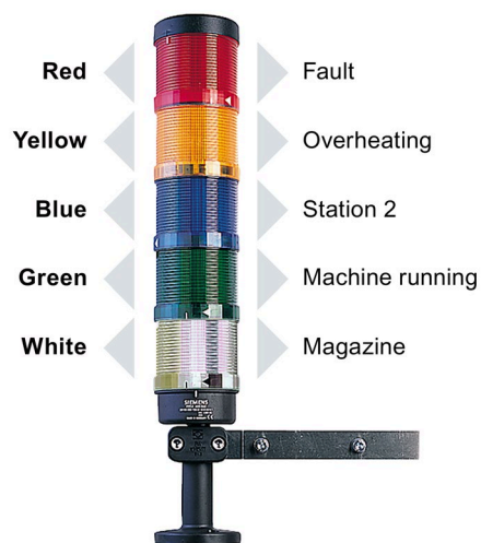
Figure 10-7 Example of Siemens 8WD4 signal column
