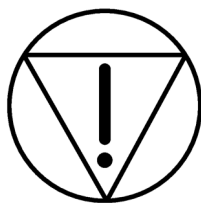
Figure 10-11 Symbol for EMERGENCY STOP
