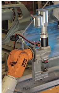
Figure 11-15 Cable routing to moving elements of the machine
