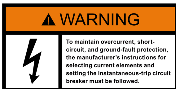
Figure 13-13 Example of warning notice for Instantaneous trip circuit breaker
