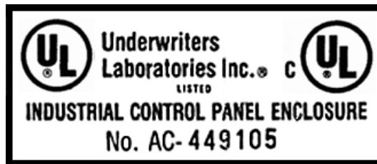
Figure 5-19 Label for a UL-tested empty industrial control panel enclosure
