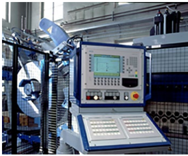
Figure 10-10 Example of operator station with EMERGENCY STOP
