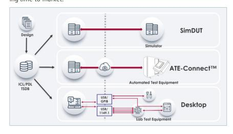
The Tessent SiliconInsight interactive environments: Test pattern validation before first silicon, debug of IJTAG devices on ATE, and debug using a local desktop environment.
